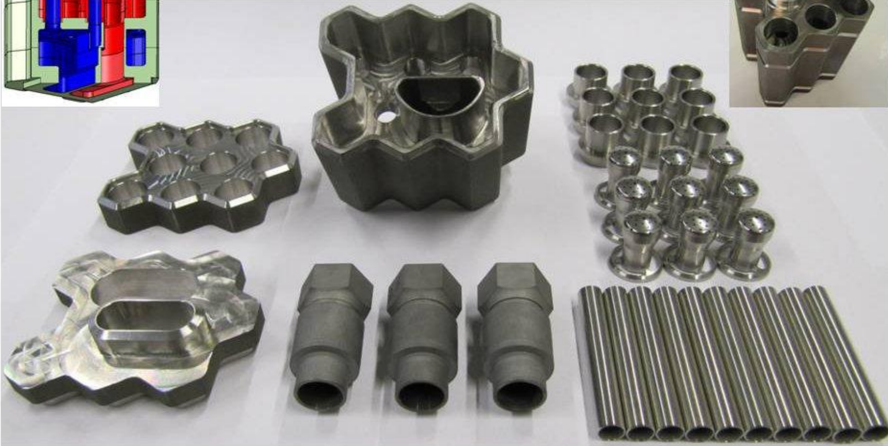
Figure 6: Manufacturing of the 9-finger module for the Helium cooled divertor developed in KIT [Norajitra].
